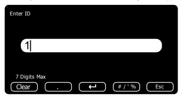
2. Use the keypad on the ZM615 to enter up to seven digits for the ID. When you have entered the ID, press the **ENTER** key and the following is displayed ...
