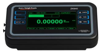
Checkweighing screen showing under weight
