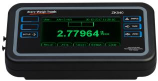
Checkweighing screen showing over weight
