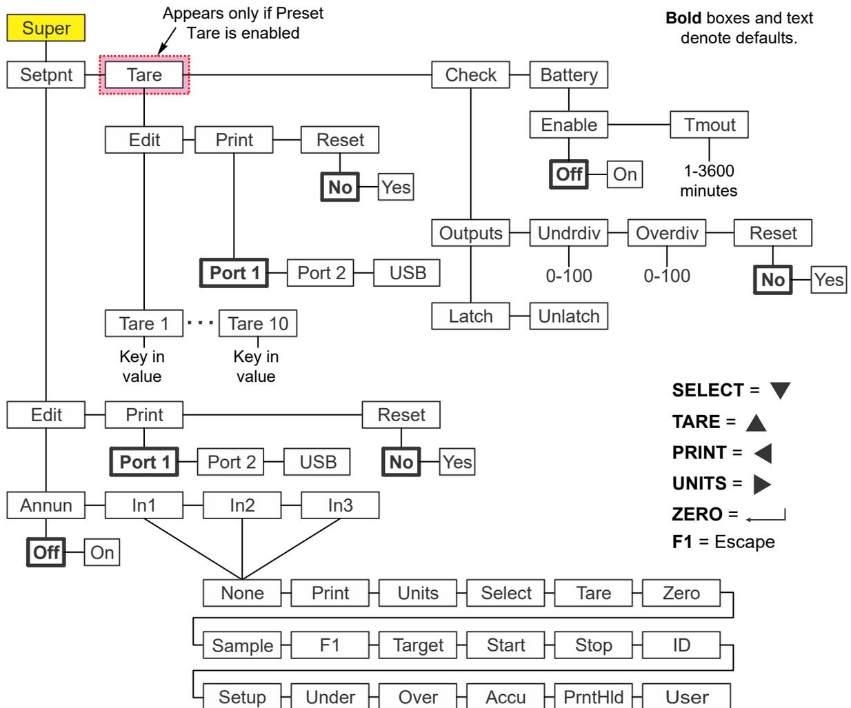
Figure 7.4 Supervisor menu for the Checkweighing application
