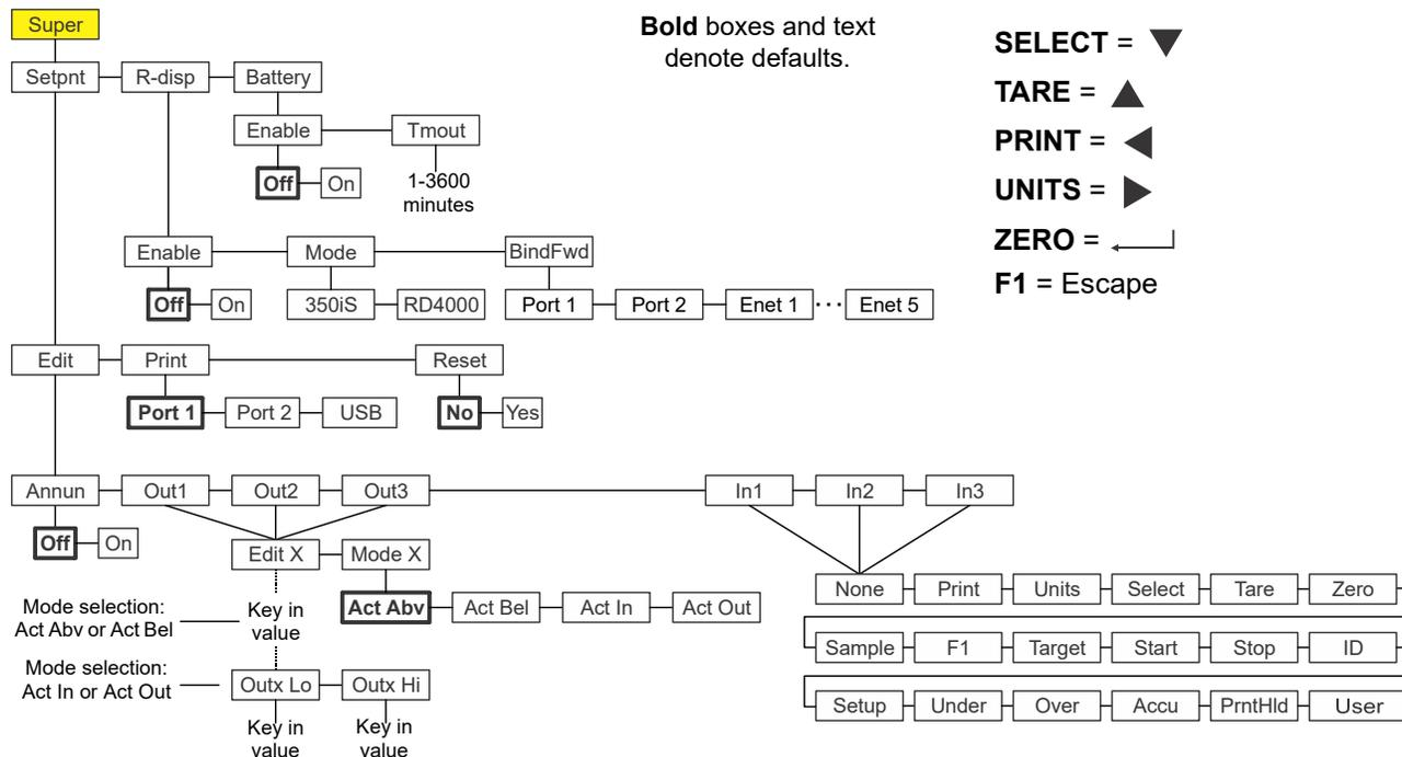
Figure 7.7 Supervisor menu for the Remote Display application
