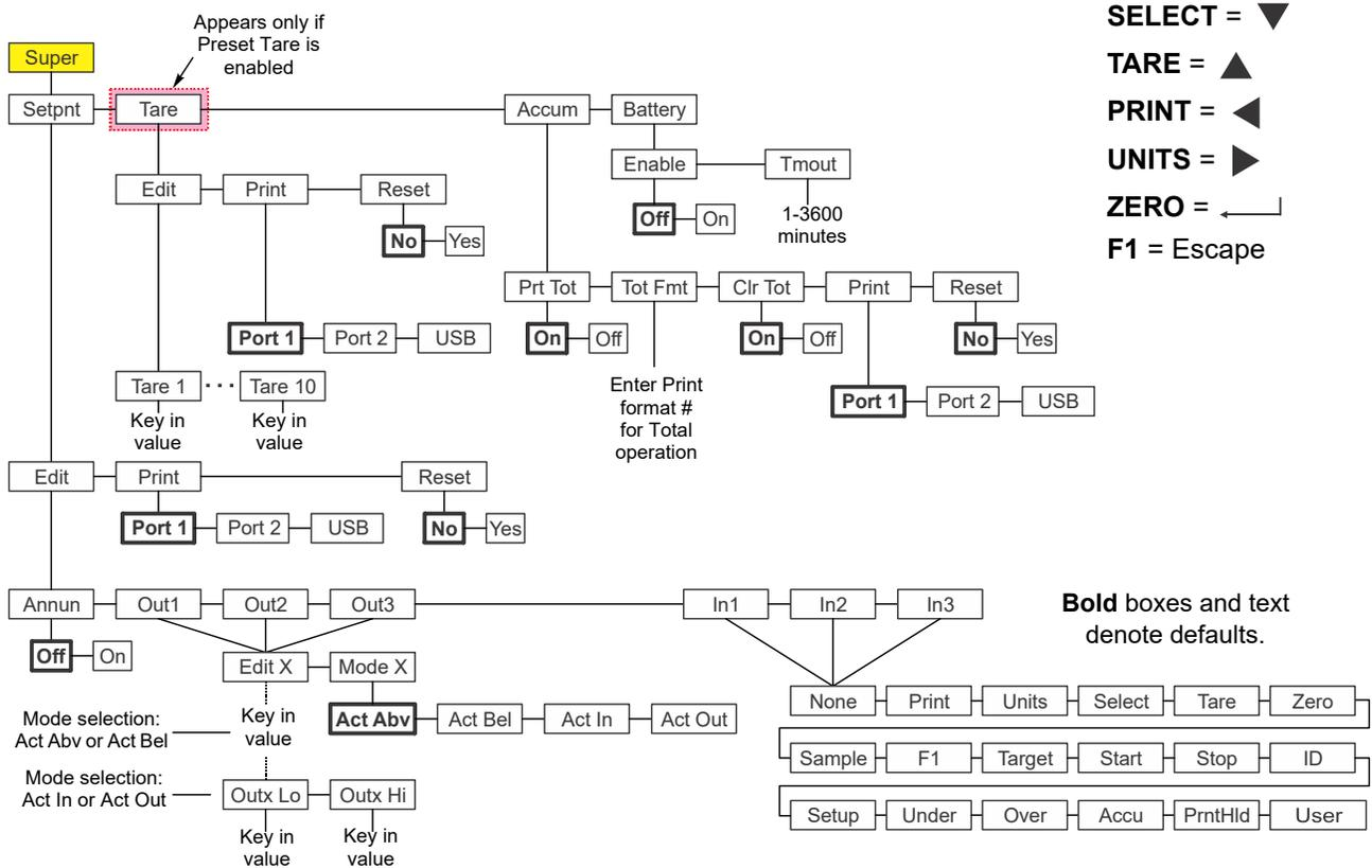
Figure 7.2 Supervisor menu for the Accumulator application
