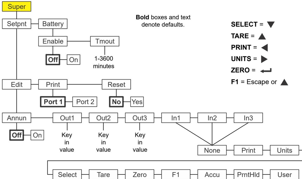
Figure 8.1 Supervisor menu for the General Weighing application
