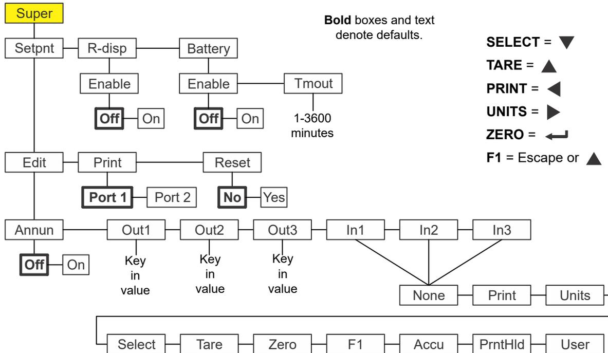
Figure 8.7 Supervisor menu for the Remote Display application
