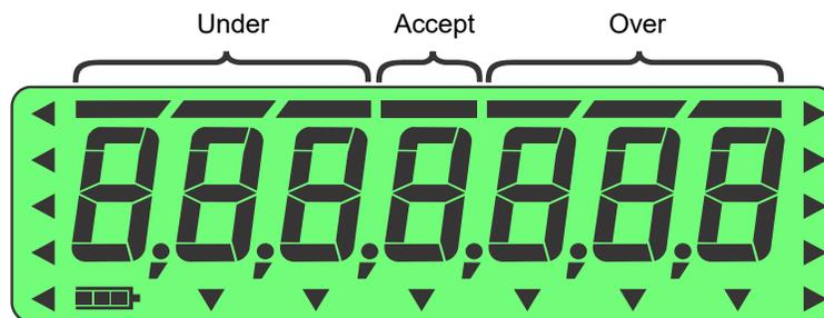
Figure 3.1 Checkweighing bargraph
