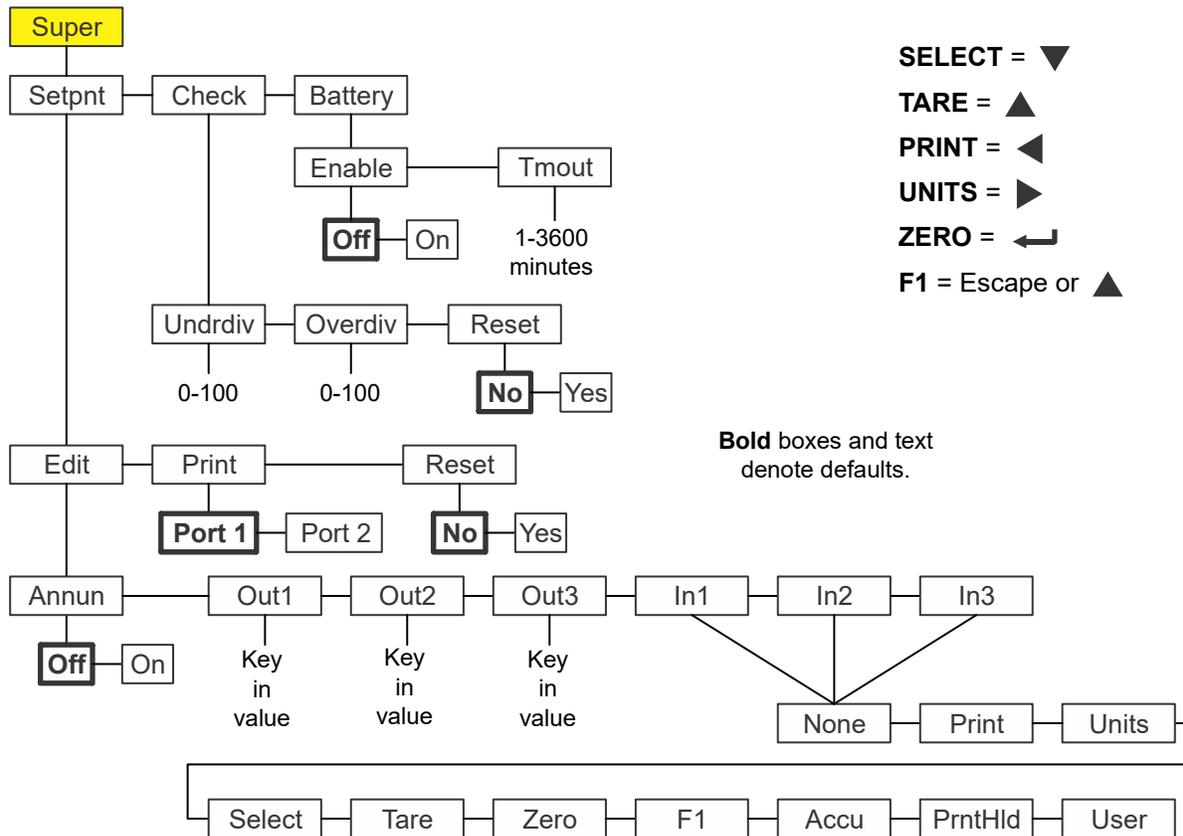
Figure 8.4 Supervisor menu for the Checkweighing application
