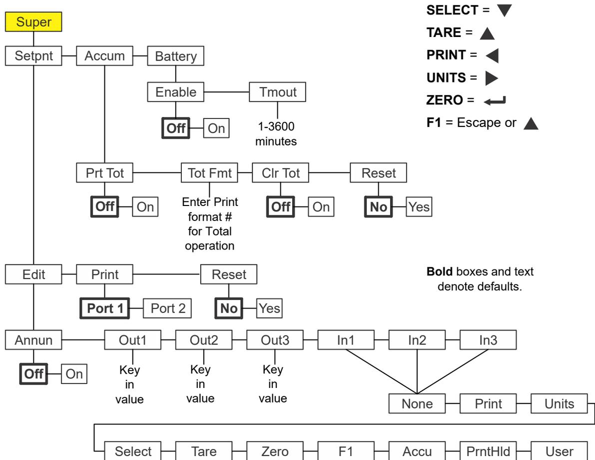
**Figure 8.2 Supervisor menu for the Accumulator application**
