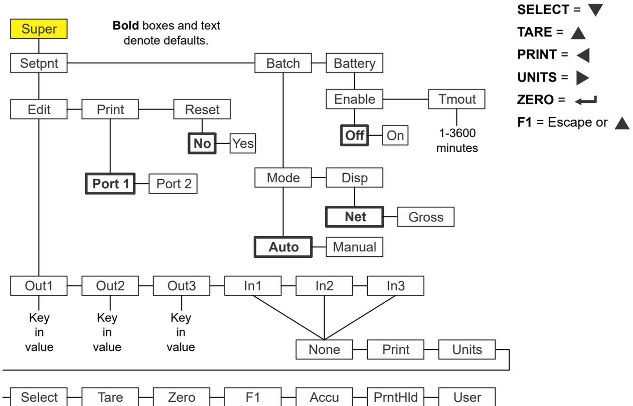
Figure 8.5 Supervisor menu for the Batching application
