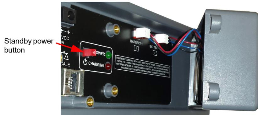
**Figure 2.8 Battery pack connections**
