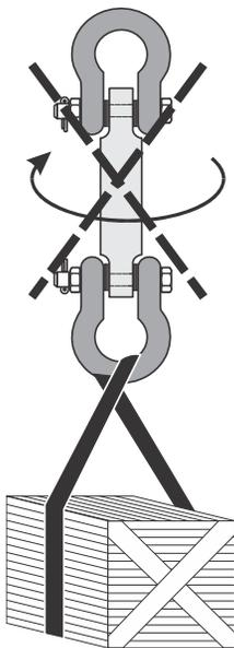
Do not torque, bend or side-load.
