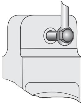
Use only with a pin of the same diameter and hardness as the original factory equipment.
