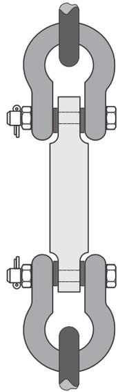
**Be sure fixturing does not bind between the body of the EDjr and the shackle!**
