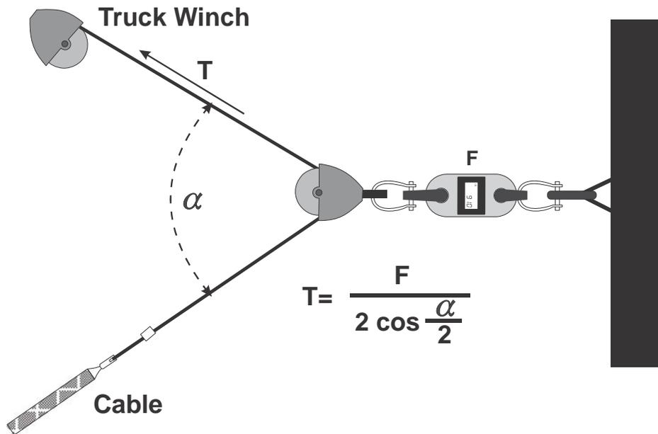
The setup shown above will give you an approximate tension reading. This can vary from actual tension due to variables in equipment and environment.
