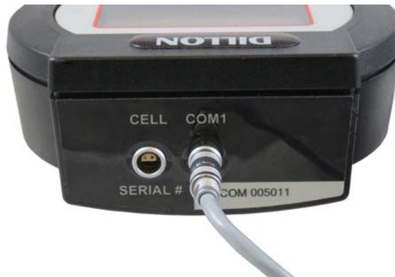
**Figure 2.7 External Power Supply Connection (Communicator)**
