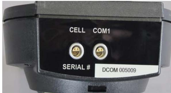
**Figure 2.6 CELL and COM1 Connectors**
