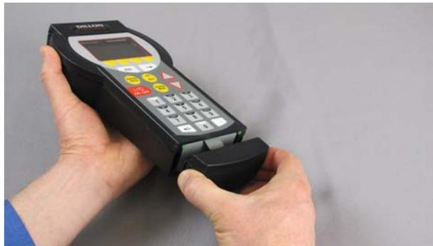
2. Press the tab of the gray battery box. The battery box will pop out slightly. Pull on the box to remove it from the Communicator.
