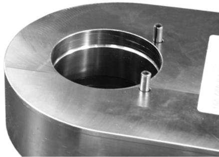
**Figure 7.3 Roll Pins Extending Above Dynamometer Body**
