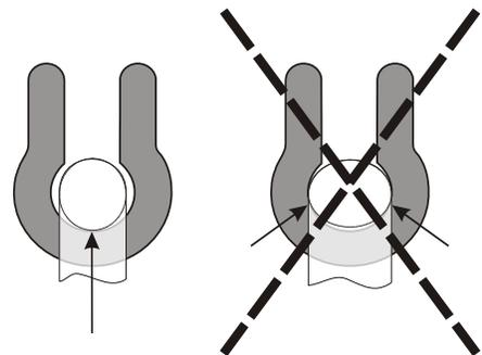
Use hardware that allows single point attachment and freedom of alignment. Do not use hardware that is undersize or restricts self-alignment. This results in poor measurement performance and possible dangerous safety conditions.
