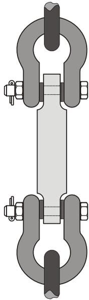
**Be sure fixturing does not bind between the body of the EDX and the shackle!**
