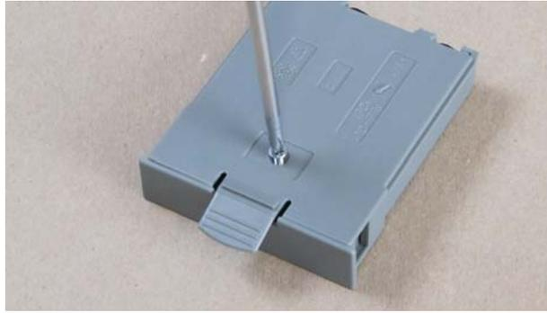
4. Remove the batteries (with a screwdriver if necessary) and replace with new AA batteries. Be sure to observe polarity when installing new batteries.
