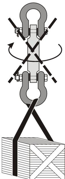
Do not torque, bend or side load.
