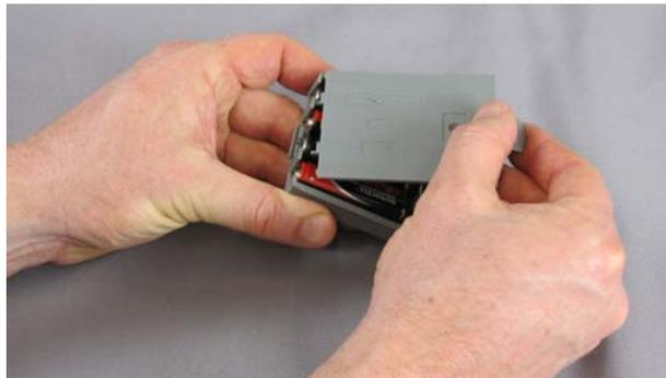
6. Push the battery holder back into the bottom of the communicator. Place the black battery cover back on the bottom of the Communicator.
