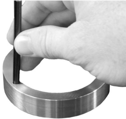
**Figure 7.2 Inserting Roll Pin**
