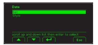
Press the up or down arrow to move the highlight and then press the Enter key to accept the choice. Press **Esc** to return to the previous screen without making a change.
