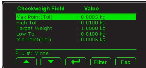
Highlight the item you want to configure for this PLUs checkweighing values, press **Enter**, key in the value and press **Enter** to accept. Press **Esc** to return to the **PLU Edit** screen.
