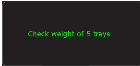
Each PLU can have a different message. The scale will display the custom message (1 line of data) until you press any key. You can set a timer to display the message after the set time has elapsed. This is ideal for reminding users to make regular sample checks
