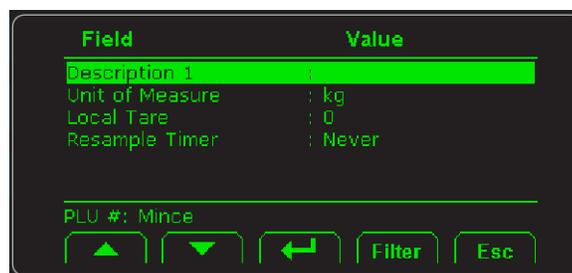
Highlight the item you want to define and press the **Enter** (← softkey). Type in a value or select from the list that appears and press the **Enter** key to accept. The **Resample Timer** item lets you set the amount of elapsed time between requests for quality assurance checks. See [QA messaging on page 18](#).
