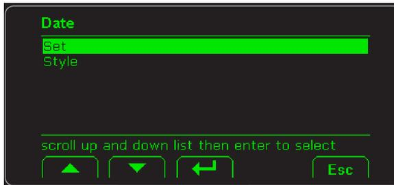
Press the **UP** (▲) or **DOWN** (▼) softkey to move the highlight and then press the **Enter** (↵) softkey to accept the highlighted choice. Press **Esc** to return to the previous screen without making a change.
