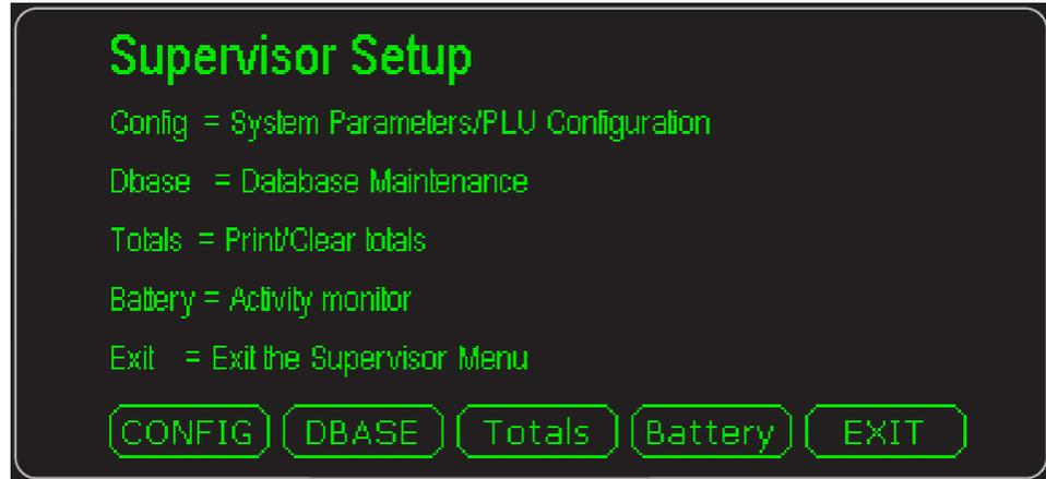
**Figure 6.2 Supervisor menu, Setup screen**
