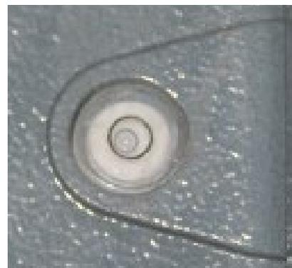
Fig. 2 Adjust feet until bubble is centered in the black circle
