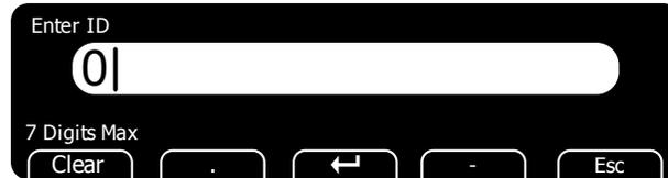
2. Use the keypad on the ZM510 to enter up to seven digits for the ID. When you have entered the ID, press the **ENTER** key and the following is displayed ...
