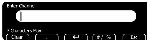
2. Key in the Channel number and press the **ENTER** key.
