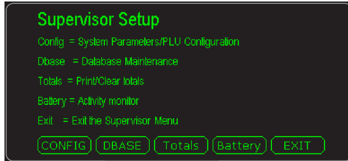
Figure 6.2 Supervisor menu, Setup screen
