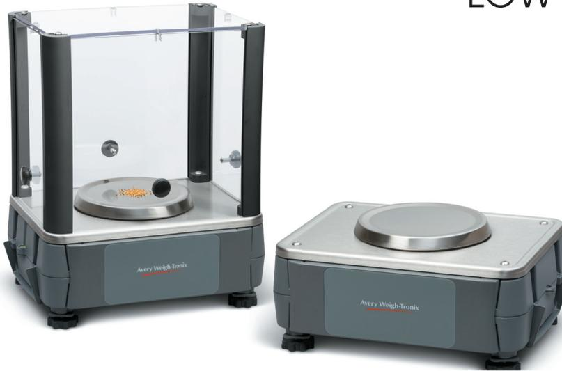
High resolution, robust bench bases designed to give balance accuracy within an industrial environment.
