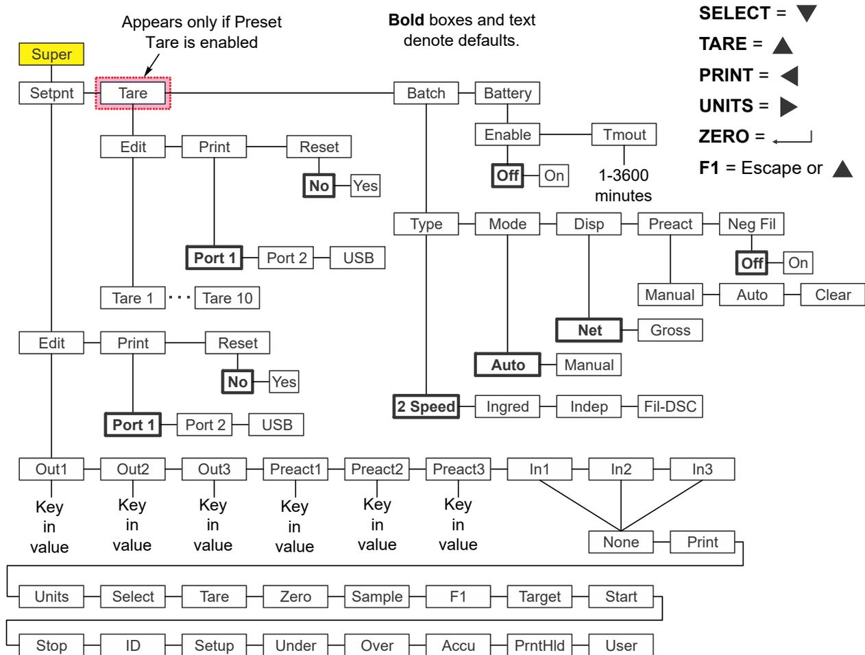
Figure 7.5 Supervisor menu for the Batching application
