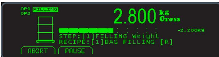
Weighing process bar showing the filling in progress and the amount still to be filled
