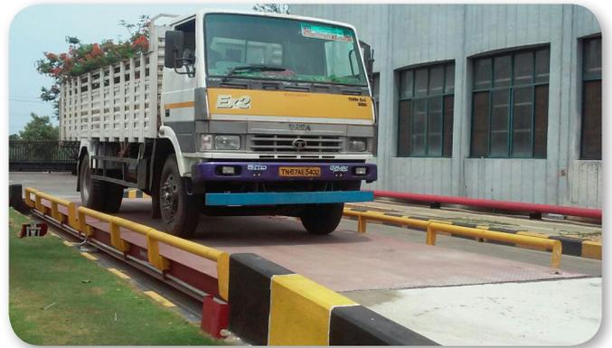
In most cases the site conditions, such as availability of space, will dictate the type of weighbridge available to you. Both surface and pit mounted weighbridges require a firm surface with load bearing capacity, the details of which will be specified in the 'Plan of Foundation' drawings provided by the weighbridge supplier.
