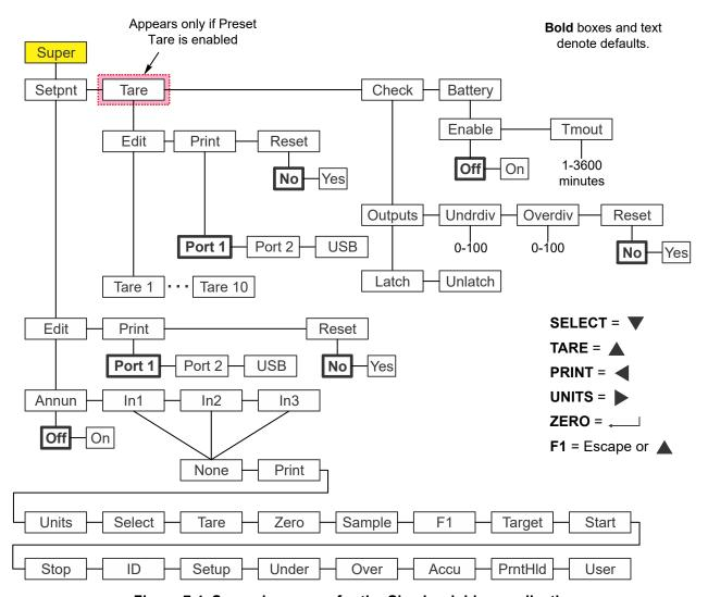
Figure 7.4 Supervisor menu for the Checkweighing application
