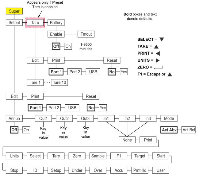
Figure 7.1 Supervisor menu for the General Weighing application
