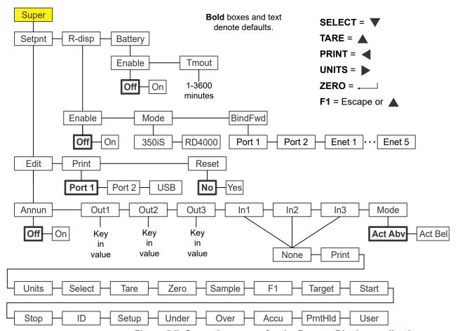
Figure 7.7 Supervisor menu for the Remote Display application
