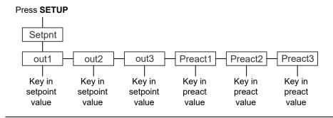
Setpoint or Preact values can be either positive or negative, up to or equal to scale capacity. See *Entering a negative number on page 14* on how to enter negative values.
