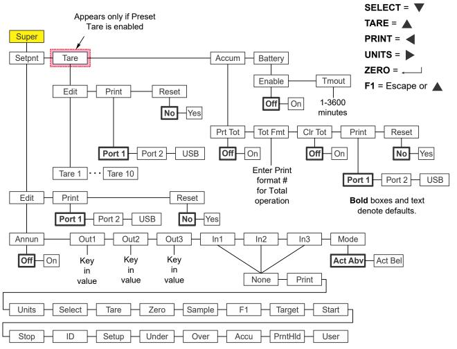
Figure 7.2 Supervisor menu for the Accumulator application
