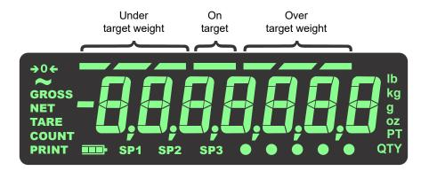
Figure 3.2 Checkweighing bargraph
