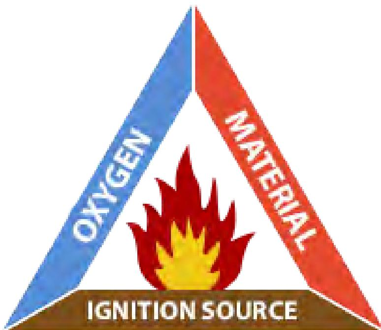
To eliminate the risk of explosion, one of the three elements of the combustion triangle must be removed.
